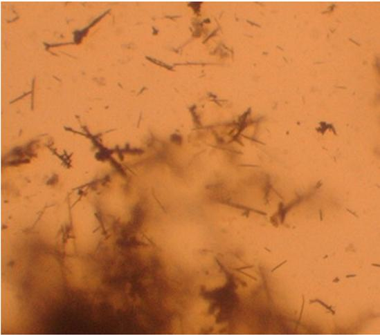
*Microscopic close-up of Pb dendrites in suspension.*
